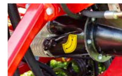
Split airflow, butterfly valve
