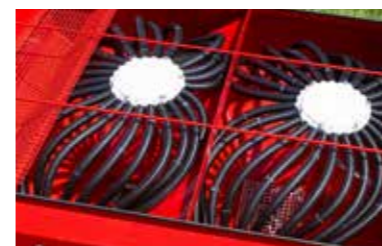
Split hopper with concealed distributor heads
