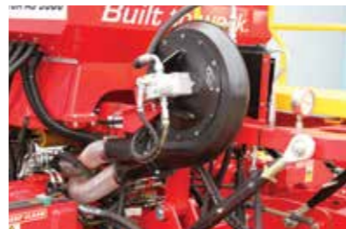
Hydraulic fan with splitter
