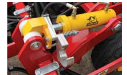
Depth adjustment on rams
