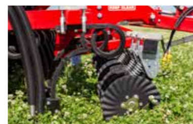
Turbo Tilth disc, tine and boot
