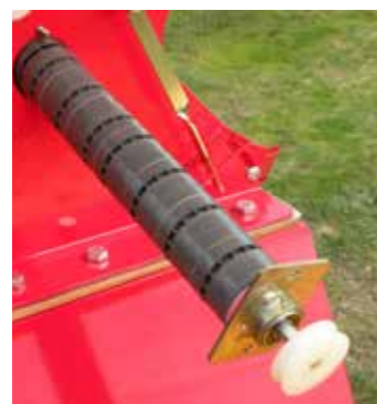
Easily changed metering cartridge
