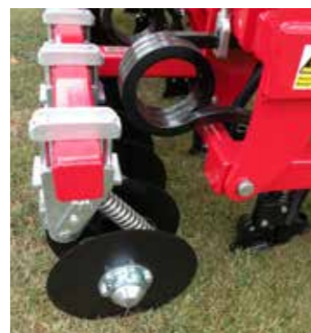
Opening disc & tine/boot/point
