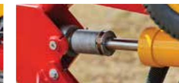
Depth adjustment on the ram
