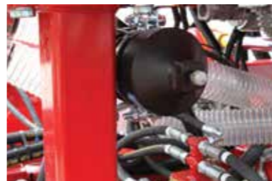
Hydraulic accumulator for holding wing pressure
