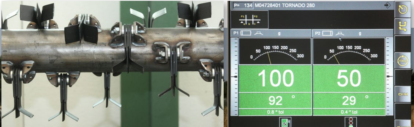
A correctly balanced rotor delivers the best possible performance and ensures lengthy implement service life.
