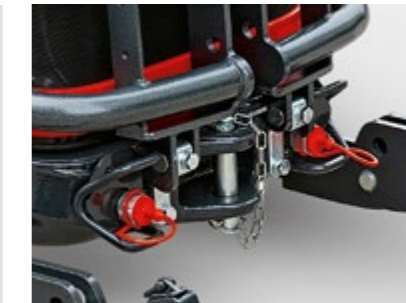
FRONT QUICK COUPLERS Hydraulic front lift complete with 3-point linkage + 1 replicated front double-acting remote (2 front quick couplers).
