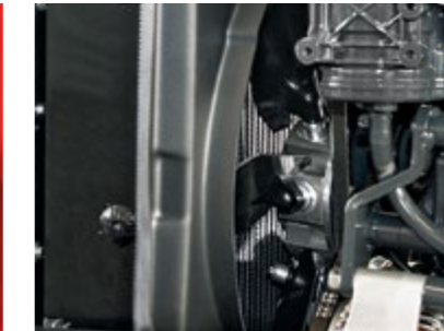
ACS (Air Clean System) Engine cooling fan with air flow reversal. Reduces the need for cleaning the front grille, ensuring more constant engine cooling.
