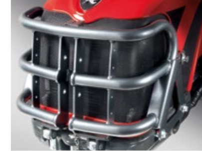
BULLBAR Tubular steel guard protecting the bodywork; integrates the third-point for the front lift.
