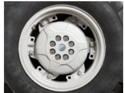
REAR CAST IRON WHEEL FLANGES Flanges that increase the weight of the tractor at the rear.
