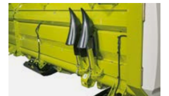
Stowage position for crop divider points during transport
