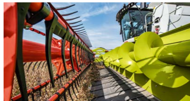
Cam-track-controlled reel with flip-over concept
