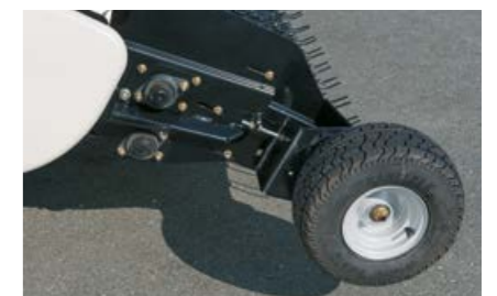
Castor guide wheels limit the depth
