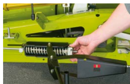
The straight belt path and the correct belt tension ensure the durability of the belts
